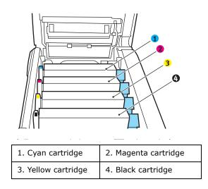
**3.** Lift each of the image drum units out of the printer and place them in a safe place away from direct sources of heat and light.
